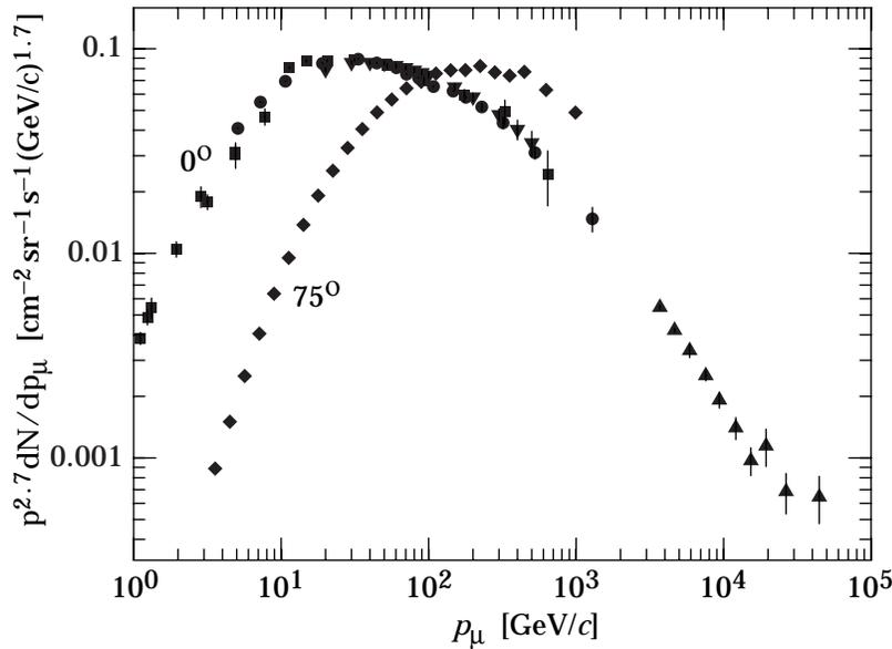
**Figure 20.4:** Spectrum of muons at  $\theta = 0^\circ$  ( $\blacksquare$  [12],  $\bullet$  [13],  $\blacktriangledown$  [14],  $\blacktriangle$  [15]), and  $\theta = 75^\circ$  ( $\blacklozenge$  [16]).
