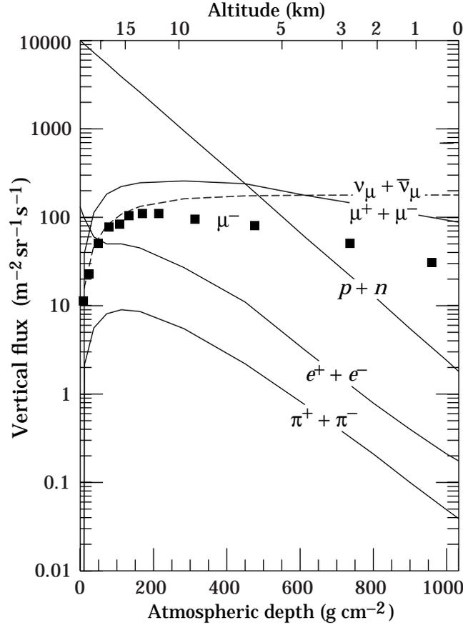
**Figure 20.3:** Vertical fluxes of cosmic rays in the atmosphere with  $E > 1$  GeV estimated from the nucleon flux of Eq. (20.2). The points show measurements of negative muons with  $E_\mu > 1$  GeV [7].
