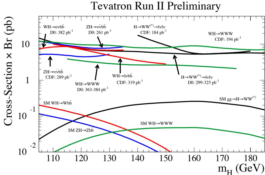
**Figure 3:** Upper bounds, obtained by the Tevatron experiments CDF and D0, for the cross-sections of event topologies motivated by Higgs boson production in the SM. The curves in the upper part represent the 95% CL experimental limits; the curves in the lower part are the SM predictions (from Ref. 30). See full-color version on color pages at end of book.
