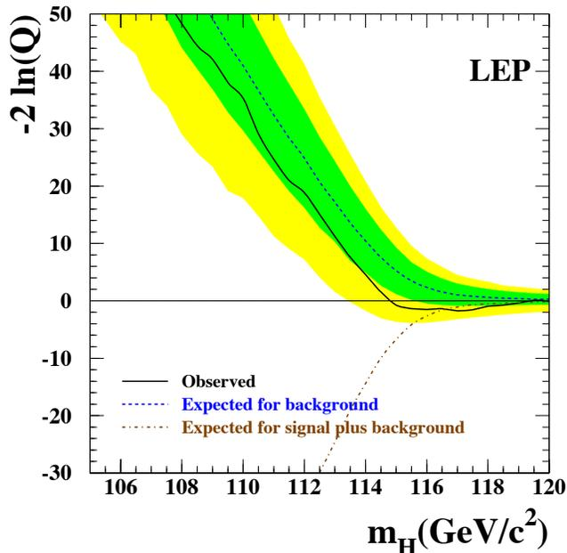
**Figure 2:** Observed (solid line), and expected behaviors of the test statistic  $-2\ln Q$  for the background (dashed line), and the signal + background hypothesis (dash-dotted line) as a function of the test mass  $m_H$ . Left: ALEPH data alone; right: LEP data combined. The dark and light shaded areas represent the 68% and 95% probability bands about the background expectation (from Ref. 27). See full-color version on color pages at end of book.
