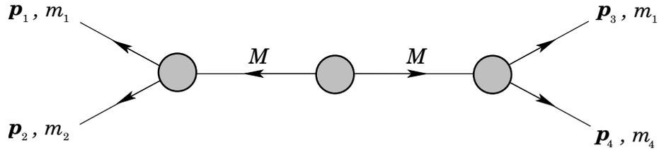
**Figure 45.9:** Definitions of variables for pair production of semi-invisible final states. Particles 1 and 3 are invisible while particles 2 and 4 are visible.
