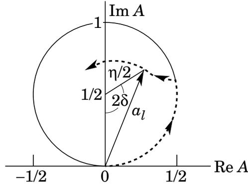
**Figure 45.7:** Argand plot showing a partial-wave amplitude  $a_{\ell}$  as a function of energy. The amplitude leaves the unitary circle where inelasticity sets in ( $\eta_{\ell} < 1$ ).
