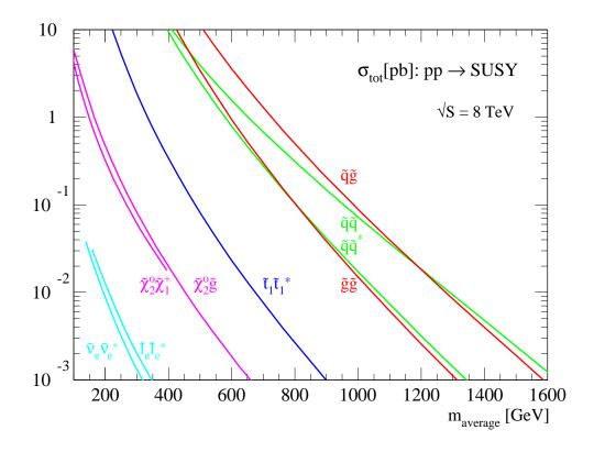
Figure 1: Cross sections for pair production of different sparticles as a function of their mass at the LHC for a center-of-mass energy of 8 TeV [52]. Typically the production cross section of colored squarks and gluinos is several orders of magnitude larger than the one for leptons or charginos. Except for the explicitly shown pair production of stops, production cross sections for squarks assumes mass degeneracy of left- and right-handed u, d, s, c and b squarks.
