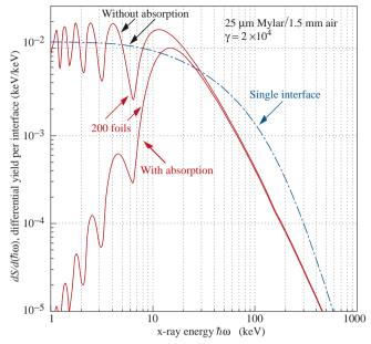
Figure 33.27: X-ray photon energy spectra for a radiator consisting of 200  $25 \,\mu\mathrm{m}$  thick foils of Mylar with 1.5 mm spacing in air (solid lines) and for a single surface (dashed line). Curves are shown with and without absorption. Adapted from Ref. 88.
