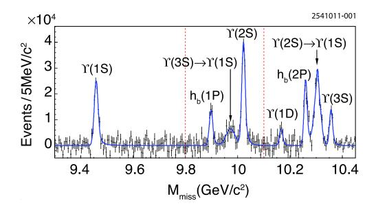
**Figure 90.1:** From Belle [18], the mass recoiling against  $\pi^+\pi^-$  pairs,  $M_{\text{miss}}$ , in  $e^+e^-$  collision data taken near the peak of the  $\Upsilon(10860)$  (*points with error bars*). The smooth combinatorial and  $K_S^0 \to \pi^+\pi^-$  background contributions have been subtracted. The fit to the various labeled signal contributions is overlaid (*curve*). Adapted from [18] with kind permission, copyright (2011) The American Physical Society.
