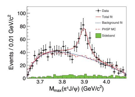
**Figure 90.3:**  $J/\psi\pi$  invariant mass distributions from BES-III [49]  $e^+e^-$  collision data taken near the peak of the Y(4260). Adapted from [49] with kind permission, copyright (2013) The American Physical Society.
