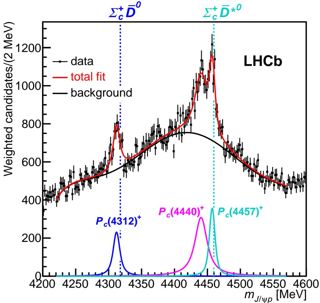
Figure 85.2: Fit to the  $J/\psi p$  mass distribution, in which events were weighted to suppress  $\Lambda^* \rightarrow pK^-$  backgrounds, of three Breit-Wigner functions and a sixth-order polynomial background. This fit was used to determine the central values of the masses and widths of the  $P_c^+$  states reported by LHCb. The mass thresholds for the  $\Sigma_c^+ \bar{D}^0$  and  $\Sigma_c^+ \bar{D}^{*0}$  final states are superimposed.
