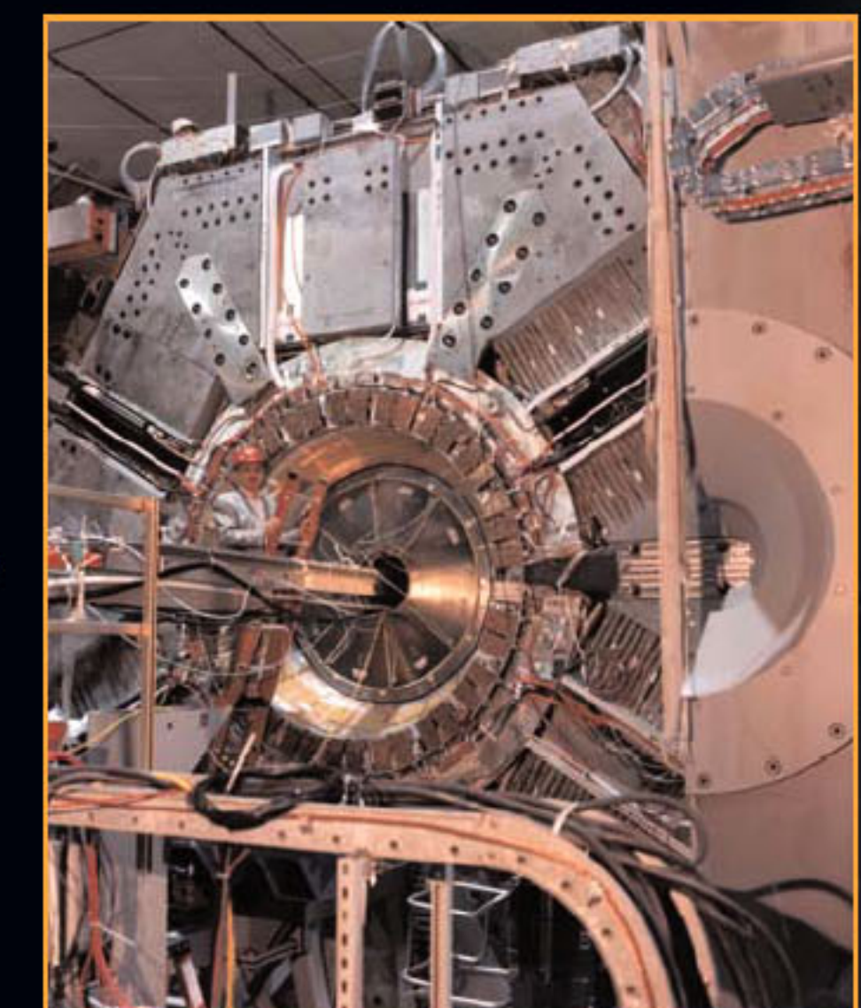
The calorimeter of the BaBar detector at the Stanford Linear Accelerator Center (SLAC). This end view shows some of the concentric layers used to track particles.
