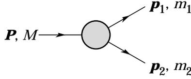
**Figure 35.1:** Definitions of variables for two-body decays.
