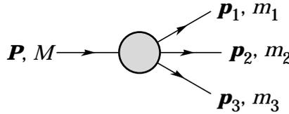
**Figure 35.2:** Definitions of variables for three-body decays.
