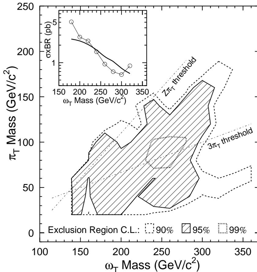
**Figure 2:** 95% CL exclusion region [17] for a light techniomuon decaying to  $\gamma$  and a  $\pi_T$ , and in which the  $\pi_T$  decays to two jets including at least one  $b$  quark. (Inset: cross section limit for  $m_{\pi_T} = 120$  GeV.)
