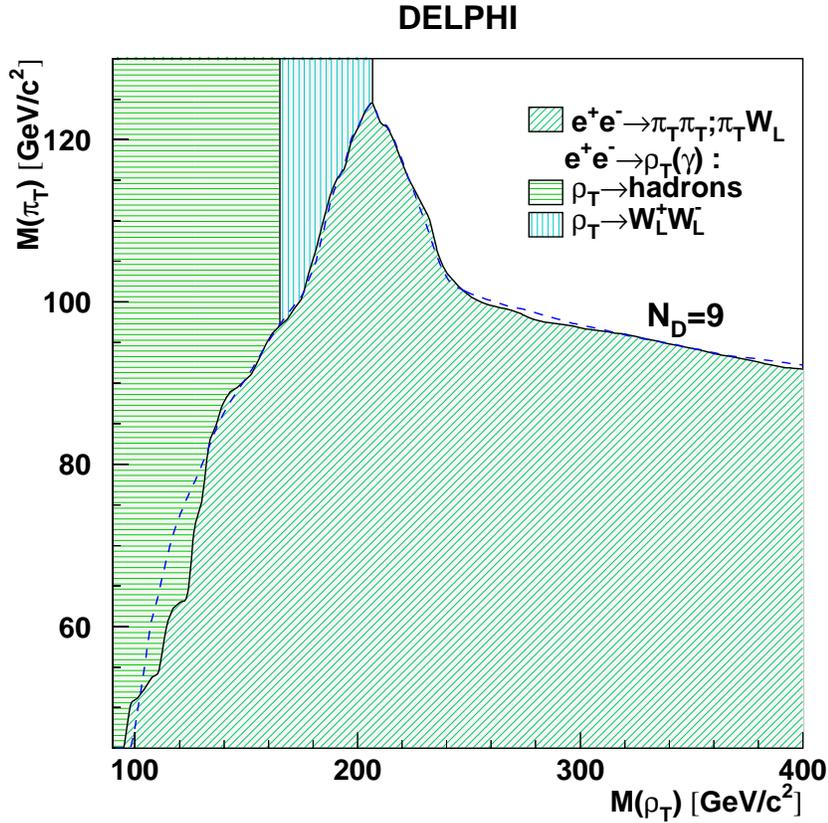
**Figure 4:** 95% CL exclusion region [20] in the technirho-technipion mass plane obtained from searches by the DELPHI collaboration at LEP 2, for nine technifermion doublets. The dashed line shows the expected limit for the 4-jet analysis.
