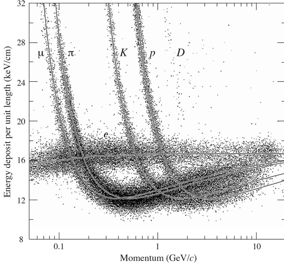
**Figure 28.8:** PEP4/9-TPC energy-deposit measurements (185 samples @8.5 atm Ar-CH<sub>4</sub> 80–20%) in multihadron events. The electrons reach a Fermi plateau value of 1.4 times the most probably energy deposit at minimum ionization. Muons from pion decays are separated from pions at low momentum;  $\pi/K$  are separated over all momenta except in the cross-over region. (Low-momentum protons and deuterons originate from hadron-nucleus collisions in inner materials such as the beam pipe.)
