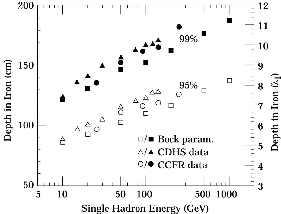
**Figure 28.13:** Required calorimeter thickness for 95% and 99% hadronic cascade containment in iron, on the basis of data from two large neutrino detectors and the parameterization of Bock *et al.* [124].
