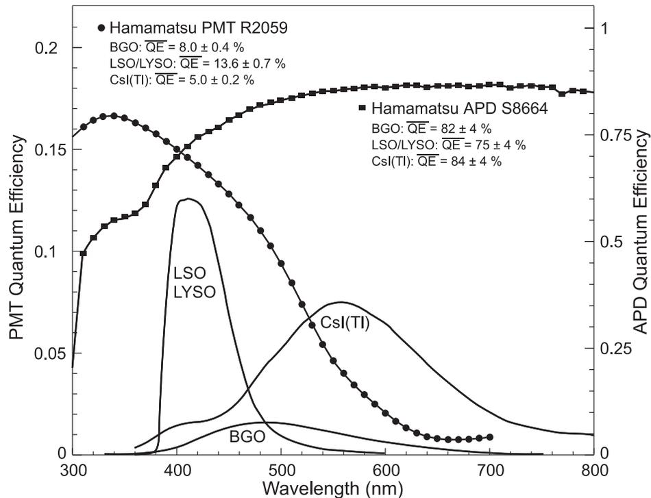
**Figure 28.2:** The quantum efficiencies of two photodetectors, a Hamamatsu R2059 PMT with bi-alkali cathode and a Hamamatsu S8664 avalanche photodiode (APD), are shown as a function of wavelength. Also shown in the figure are emission spectra of three crystal scintillators, BGO, LSO and CsI(Tl), and the numerical values of the emission weighted quantum efficiency. The area under each emission spectrum is proportional to crystal's light yield.
