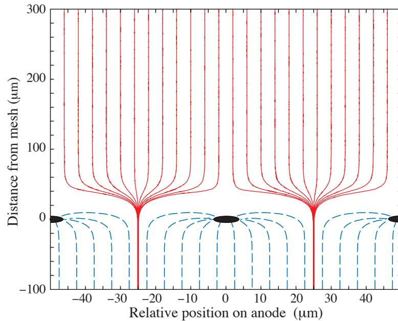
**Figure 28.6:** GARFIELD simulation of the electron (solid) and positive ion (dashed) drift lines in a Micromegas avalanche region. Drifting electrons are funneled through the mesh and spread across the anode surface by diffusion (not included). Most positive ions produced in the gap near the anode surface drift back to the Micromegas mesh.
