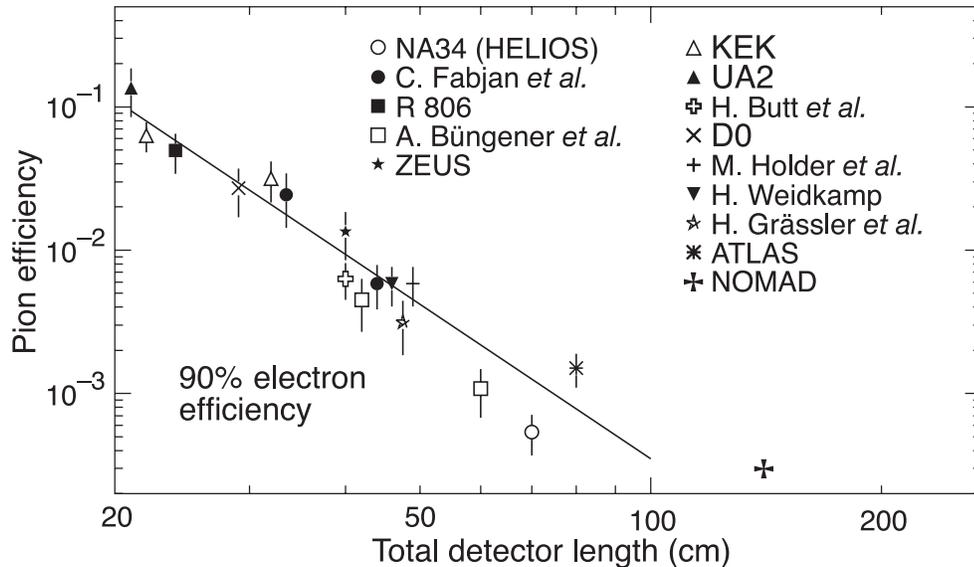
**Figure 28.3:** Pion efficiency measured (or predicted) for different TRDs as a function of the detector length for a fixed electron efficiency of 90%. The experimental data are directly taken or extrapolated from references [77–89,70] (NA34 to NOMAD).
