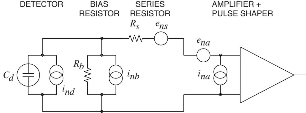
**Figure 28.11:** Equivalent circuit for noise analysis.
