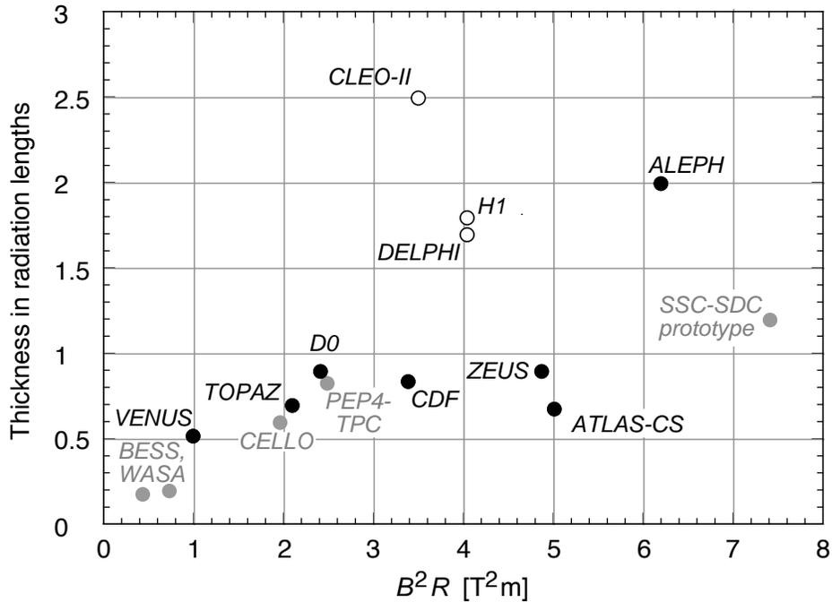
**Figure 28.15:** Magnet wall thickness in radiation length as a function of  $B^2R$  for various detector solenoids. Gray entries are for magnets not listed in Table 28.8. Open circles are for magnets not designed to be “thin.” The SSC-SDC prototype provided important R&D for LHC magnets.
