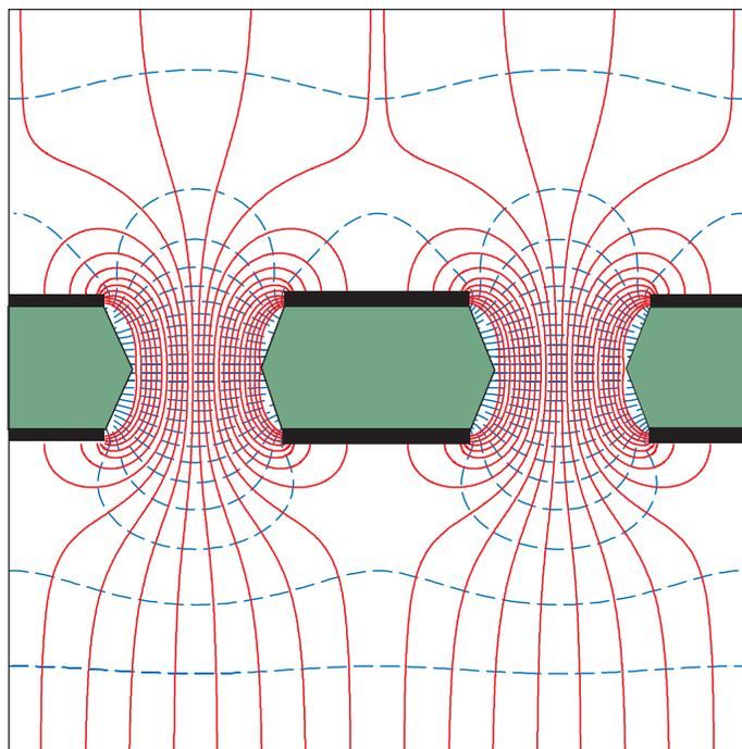
**Figure 28.5:** Detail of electric field lines (solid) and equipotentials (dashed) in the region of GEM holes. Electron transparencies are typically 100%. Most positive ions produced in the high field region within a hole drift back to the GEM's top side. Figure courtesy of F. Sauli.
