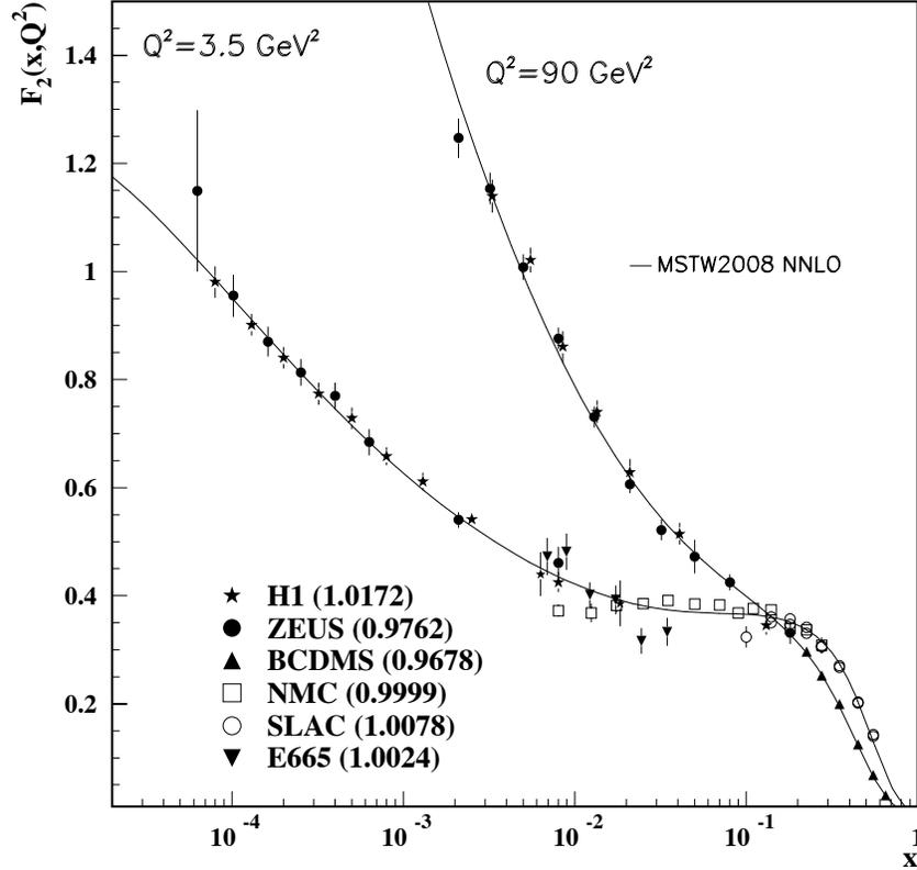
**Figure 16.2:** The proton structure function  $F_2^p$  given at two  $Q^2$  values ( $3.5 \text{ GeV}^2$  and  $90 \text{ GeV}^2$ ), which exhibit scaling at the ‘pivot’ point  $x \sim 0.14$ . See the captions in Fig. 16.7 and Fig. 16.10 for the references of the data. The various data sets have been renormalised by the factors shown in brackets in the key to the plot, which were determined in the NNLO MSTW2008 global analysis, see Table 3 of [13].
