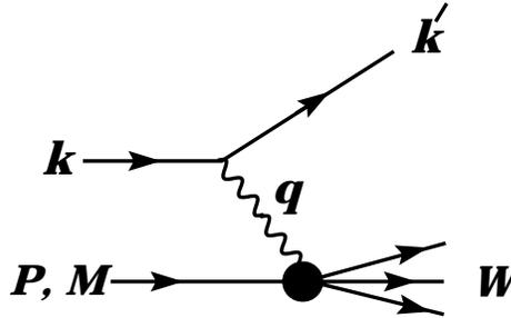
**Figure 16.1:** Kinematic quantities for the description of deep inelastic scattering. The quantities  $k$  and  $k'$  are the four-momenta of the incoming and outgoing leptons,  $P$  is the four-momentum of a nucleon with mass  $M$ , and  $W$  is the mass of the recoiling system  $X$ . The exchanged particle is a  $\gamma$ ,  $W^\pm$ , or  $Z$ ; it transfers four-momentum  $q = k - k'$  to the nucleon.
