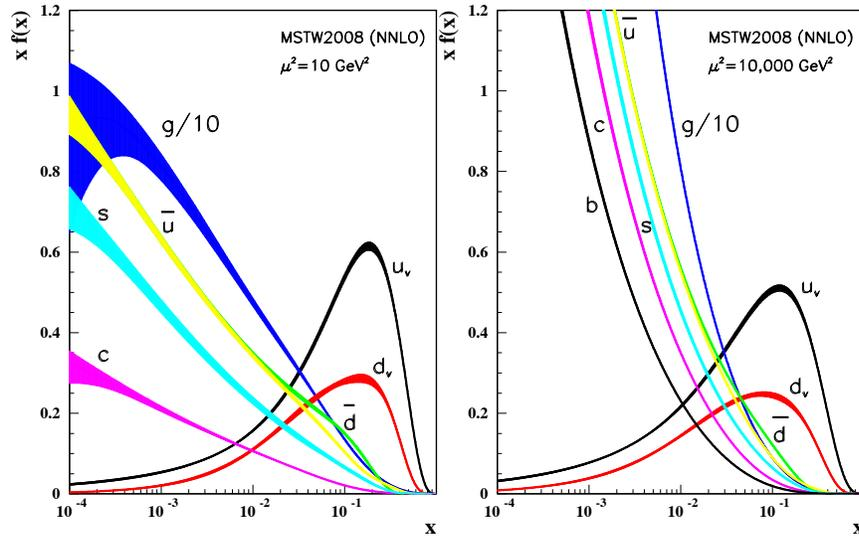
**Figure 16.4:** Distributions of  $x$  times the unpolarized parton distributions  $f(x)$  (where  $f = u_v, d_v, \bar{u}, \bar{d}, s, c, b, g$ ) and their associated uncertainties using the NNLO MSTW2008 parameterization [13] at a scale  $\mu^2 = 10 \text{ GeV}^2$  and  $\mu^2 = 10,000 \text{ GeV}^2$ .
