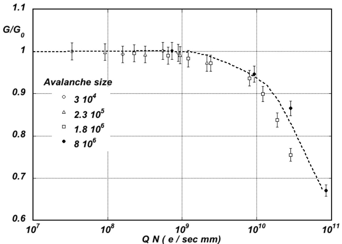
**Figure 31.8:** Charge rate dependence of normalized gas gain  $G/G_0$  (relative to zero counting rate) in proportional thin-wire detectors [80].  $Q$  is the total charge in single avalanche;  $N$  is the particle rate per wire length.
