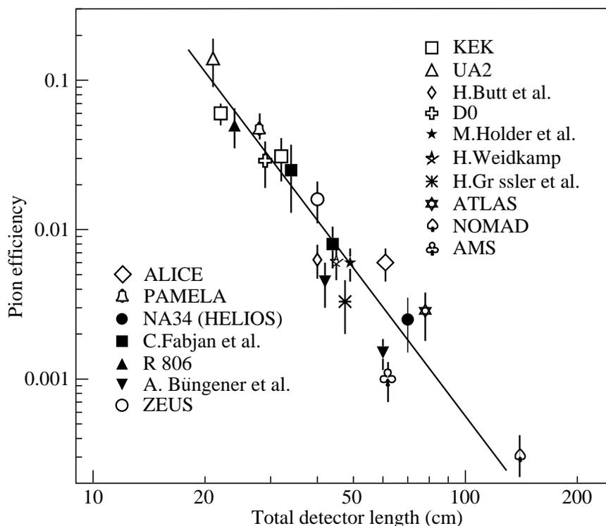
**Figure 31.16:** Pion efficiency measured (or predicted) for different TRDs as a function of the detector length for a fixed electron efficiency of 90%. The plot is taken from [106] with efficiencies of more recent detectors added [107].
