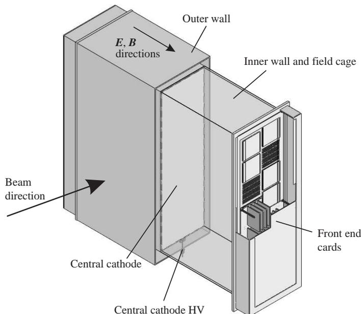
**Figure 31.14:** One of the 3 TPC modules for the near detector of the T2K experiment [103]. The drift volume is 2 m×2 m×0.8 m. Micromegas devices are used for gas amplification and readout.
