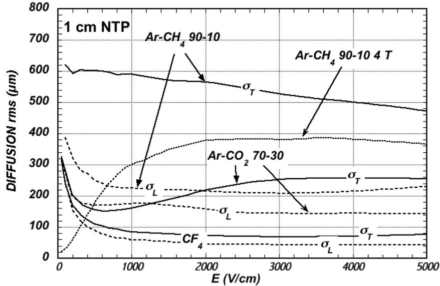
**Figure 31.5:** Electron longitudinal diffusion ( $\sigma_L$ ) (dashed lines) and transverse diffusion ( $\sigma_T$ ) (full lines) for 1 cm of drift at NTP and  $B = 0$ . The dotted line shows  $\sigma_T$  for the P10 mixture at 4 T [65].
