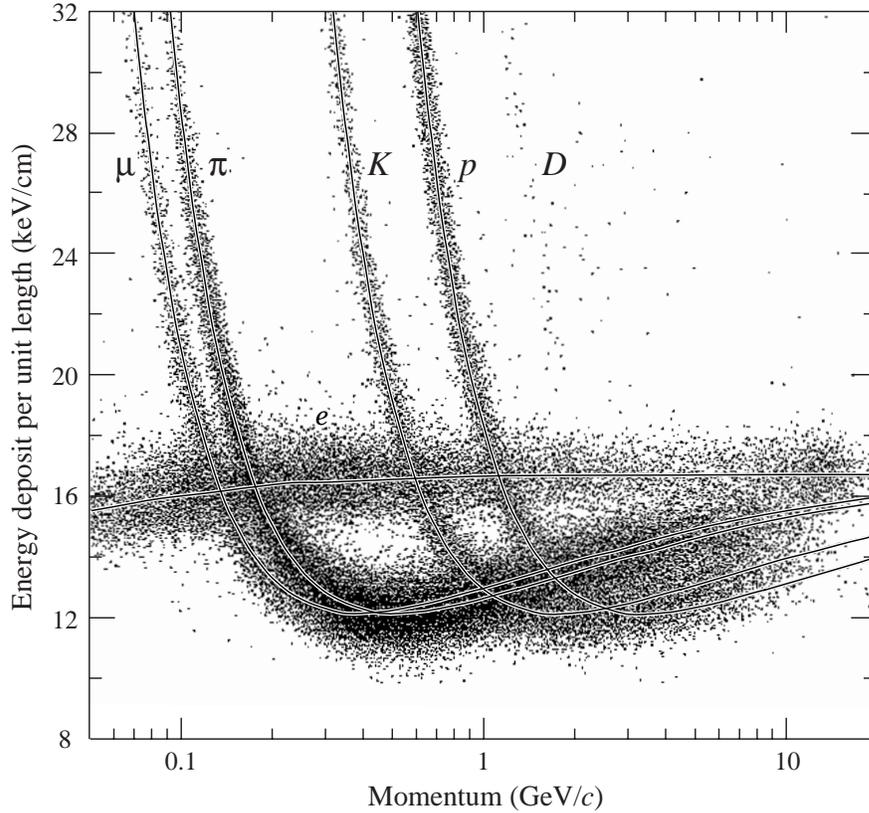
**Figure 31.15:** The PEP4/9-TPC energy deposit measurements (185 samples, 8.5 atm Ar-CH<sub>4</sub> 80:20). The ionization rate at the Fermi plateau (at high  $\beta$ ) is 1.4 times that for the minimum at lower  $\beta$ . This ratio increases to 1.6 at atmospheric pressure.
