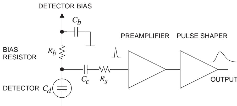
**Figure 31.18:** Typical detector front-end circuit.
