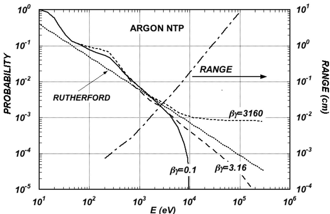
**Figure 31.3:** Probability of single collisions in which released electrons have an energy  $E$  or larger (left scale) and practical range of electrons in Ar/CH<sub>4</sub> (P10) at NTP (dot-dashed curve, right scale) [60].
