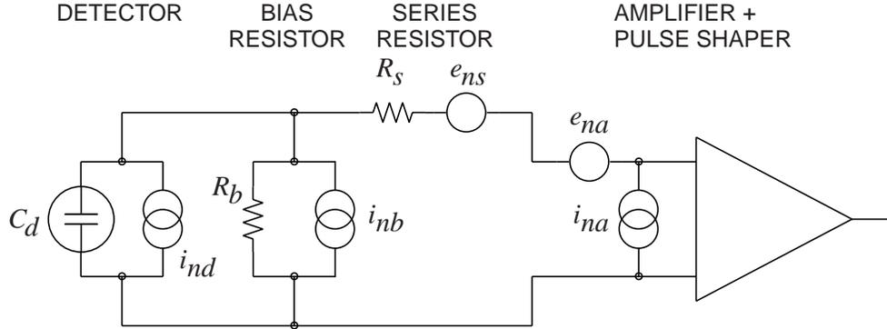
**Figure 31.19:** Equivalent circuit for noise analysis.
