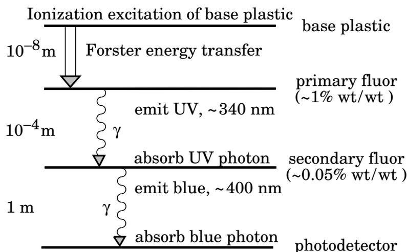
**Figure 31.1:** Cartoon of scintillation “ladder” depicting the operating mechanism of organic scintillator. Approximate fluor concentrations and energy transfer distances for the separate sub-processes are shown.
