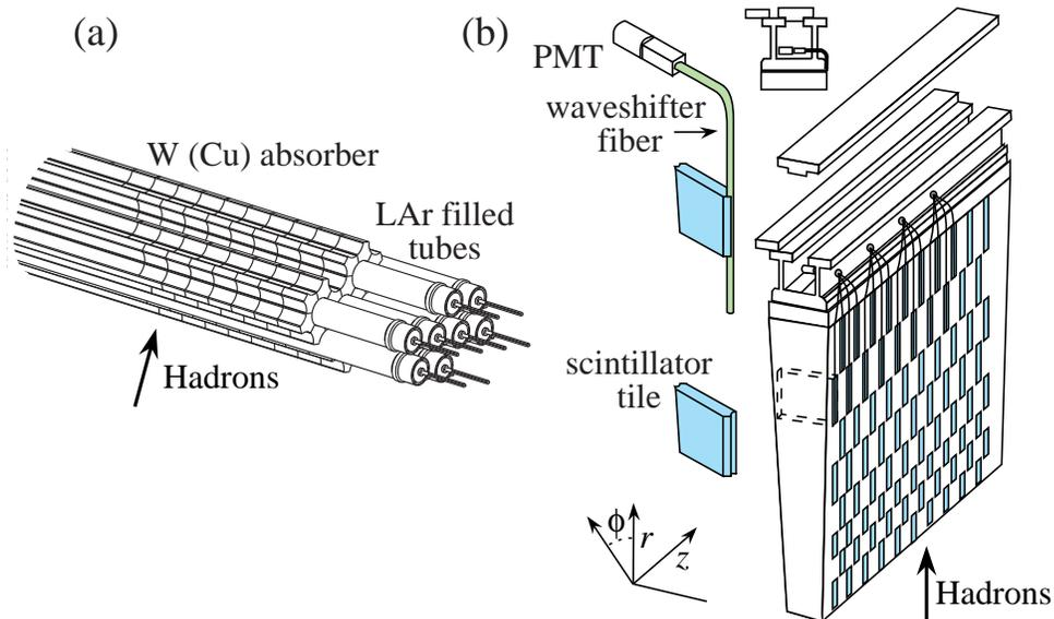
**Figure 31.22:** (a) ATLAS forward hadronic calorimeter structure (FCal2, 3). Tubes containing LAr are embedded in a mainly tungsten matrix. (b) ATLAS central calorimeter wedge; iron with plastic scintillator tile with wavelength-shifting fiber readout.
