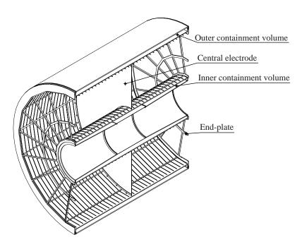
**Figure 31.13:** The ALICE TPC shown in a cutaway view [102]. The drift volume is 5 m long with a 5 m diameter. Gas amplification is provided by planes of anode wires.
