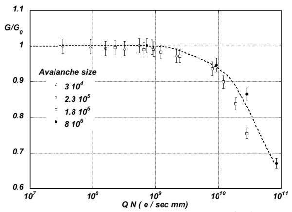
**Figure 31.8:** Charge rate dependence of normalized gas gain  $G/G_0$  (relative to zero counting rate) in proportional thin-wire detectors [80]. Q is the total charge in single avalanche; N is the particle rate per wire length.
