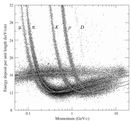
**Figure 31.15:** The PEP4/9-TPC energy deposit measurements (185 samples, 8.5 atm Ar-CH<sub>4</sub> 80:20). The ionization rate at the Fermi plateau (at high  $\beta$ ) is 1.4 times that for the minimum at lower  $\beta$ . This ratio increases to 1.6 at atmospheric pressure.
