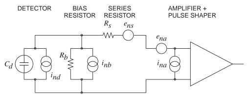
Figure 31.19: Equivalent circuit for noise analysis.
