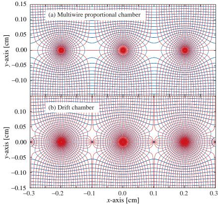
Figure 31.7: Electric field lines and equipotentials in (a) a multiwire proportional chamber and (b) a drift chamber.
