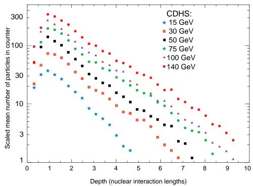
Figure 31.23: Mean profiles of  $\pi^+$  (mostly) induced cascades in the CDHS neutrino detector [143].
