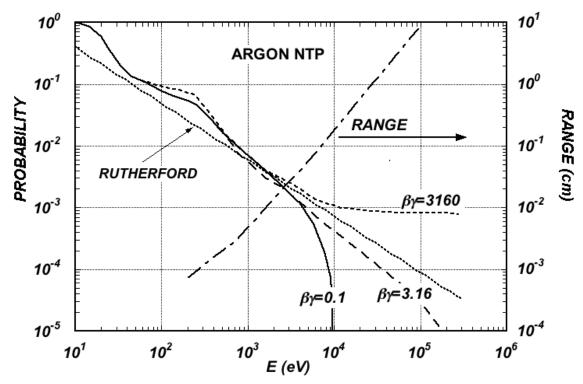
**Figure 31.3:** Probability of single collisions in which released electrons have an energy E or larger (left scale) and practical range of electrons in Ar/CH<sub>4</sub> (P10) at NTP (dot-dashed curve, right scale) [60].
