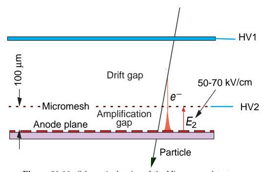
Figure 31.11: Schematic drawing of the Micromegas detector.
