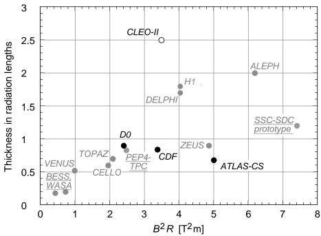
Figure 31.25: Magnet wall thickness in radiation length as a function of  $B^2R$  for various detector solenoids. Gray entries are for magnets no longer in use, and entries underlined are not listed in Table 31.9. Open circles are for magnets not designed to be "thin." The SSC-SDC prototype provided important R&D for LHC magnets.
