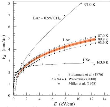
Figure 31.24: Drift velocity of free electrons as a function of electric field strength for LAr [146], LAr + 0.5% CH<sub>4</sub> [148] and LXe [147]. The average temperatures of the liquids are indicated. Results of a fit to an empirical function [152] are superimposed. In case of LAr at 91 K the error band for the global fit [146] including statistical and systematic errors as well as correlations of the data points is given. Only statistical errors are shown for the individual LAr data points.
