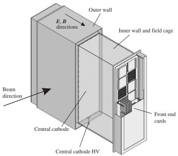
Figure 31.14: One of the 3 TPC modules for the near detector of the T2K experiment [103]. The drift volume is  $2 \text{ m} \times 2 \text{ m} \times 0.8 \text{ m}$ . Micromegas devices are used for gas amplification and readout.
