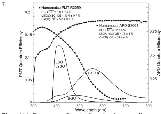
Figure 31.2: The quantum efficiencies of two photodetectors, a Hamamatsu R2059 PMT with bi-alkali cathode and a Hamamatsu S8664 avalanche photodiode (APD), are shown as a function of wavelength. Also shown in the figure are emission spectra of three crystal scintillators, BGO, LSO and CsI(Tl), and the numerical values of the emission weighted quantum efficiencies. The area under each emission spectrum is proportional to crystal's light yield.
