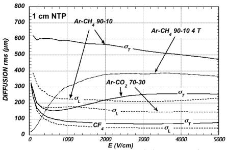
**Figure 31.5:** Electron longitudinal diffusion  $(\sigma_L)$  (dashed lines) and transverse diffusion  $(\sigma_T)$  (full lines) for 1 cm of drift at NTP and B=0. The dotted line shows  $\sigma_T$  for the P10 mixture at 4 T [65].
