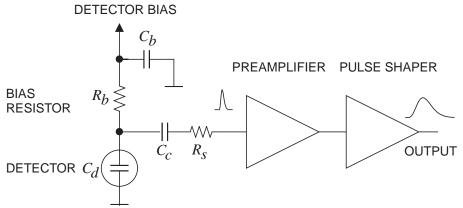
Figure 31.18: Typical detector front-end circuit.
