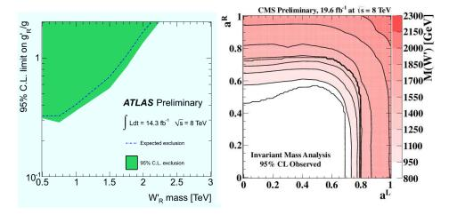
**Figure 2:** 95% CL upper limits on W' couplings using the  $t\bar{b}$  and  $\bar{t}b$  final states, assuming that the diagonal couplings are generation independent. Left panel: ATLAS [23] limit on  $C_{q_{11}}^R/g$ . Right panel: CMS [24] limit on  $M_{W'}$  as contours in the  $C_{q_{11}}^R/g - C_{q_{11}}^L/g$  plane.
