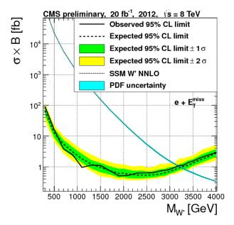
Figure 1: 95% CL limit on  $\sigma(pp \to W'X) \times B(W' \to e\nu)$  from CMS [16]. The theoretical prediction (dotted line) is for  $C_q^R = gV_{\text{CKM}}, C_l^R = g,$   $C_q^L = C_l^L = 0.$
