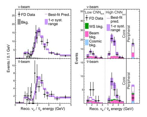
**Figure 14.6:** Reconstructed neutrino energy distributions from the NOvA far detector [122]. Top plots are for neutrino beam mode, and bottom plots are for antineutrino beam mode. Left: muon-type candidates. Right: electron-type candidates, split into a low and high purity sample as well as the event counts in the peripheral sample which occurred near the edge of the detector.
