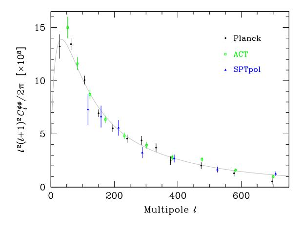
**Figure 29.6:** Power spectrum measurements for CMB lensing, including selected results from *Planck*, ACT, and SPT. The quantity plotted is the (dimensionless) potential power spectrum, scaled by  $\ell^2(\ell+1)^2$  and multiplied by a factor of  $10^8$  to make the numbers more manageable. Some less reliable measurements have not been plotted. The best-fit *Planck* ACDM spectrum is plotted as a gray line.
